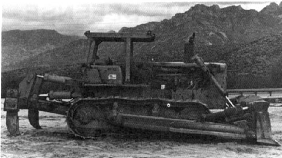
Bulldozer. Note the smoke stack (exhaust pipe).
