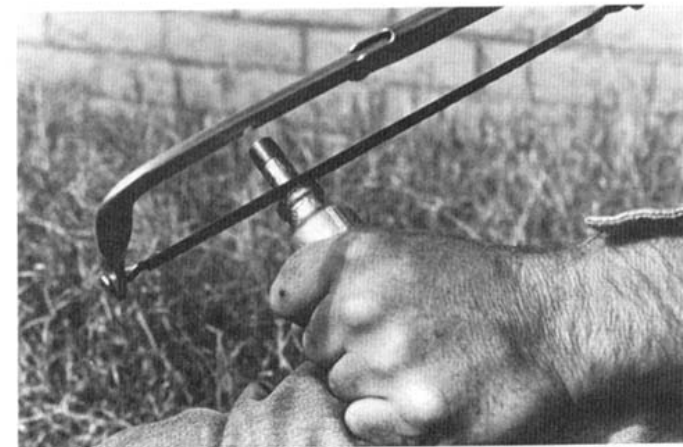
Finally, saw off the 1/4 inch nipple flush with the reducer. Your road spike driver is ready for use.
