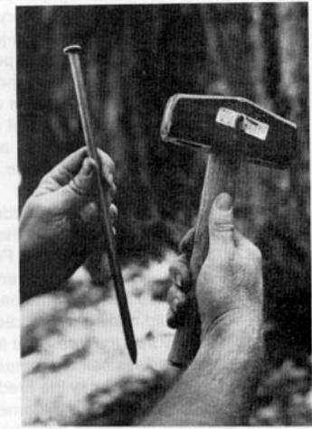
A bridge timber spike and single jack hammer for use with very large trees. Smaller spikes are fine for general use and can be driven in with a heavy standard hammer.
