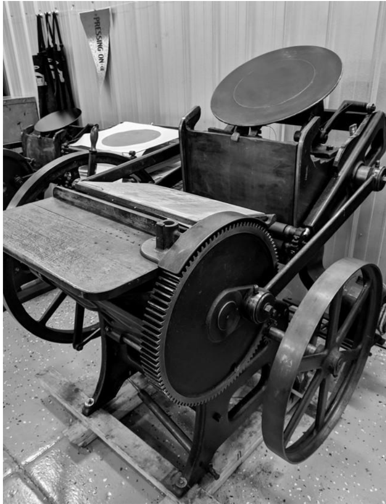
Fig. 1.1. i2 x 18 c&p platen press from Tribune Showprint, Muncie, Indiana. Photograph by Kathy Ferguson. Courtesy of Rob and Kim Miller.
