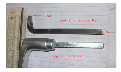
The abri, or bus-stop poster frames. But also the stand-alone rolling poster frames have a simple locking mechanism with a "key" that you can buy at a hardware store. If you are lucky, the company uses the square door handle mechanism, in some regions there is limited space so you have to make your own 8mm square bar with a bend like this one for Zeist.
