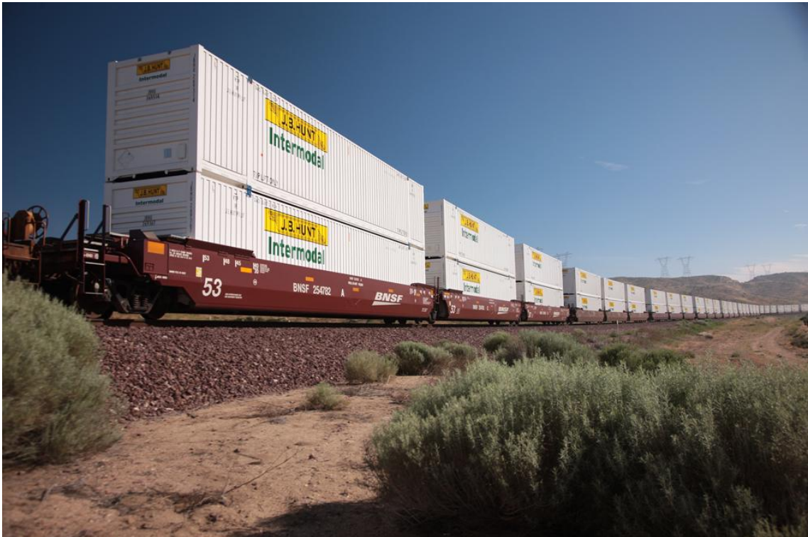
53 ft smooth cars from an IM with JB Hunt double stack cans.
