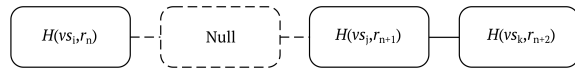
Figure 2. Where vs is the validator signature of the round identifier and r is the previous combined hashed output.
